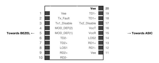
Figure 2. Transceiver Electrical Pad Layout
